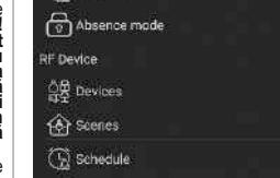
**EN - By pressing the + button, you can add a new 433.92 MHz RF socket. Enter the name of the socket (e.g. THO 1), and the type of it (Switch).**
